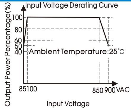
Note: ① With an input between 85 - 100VAC/850 - 900VAC, the output power must be derated as per temperature derating curves;
