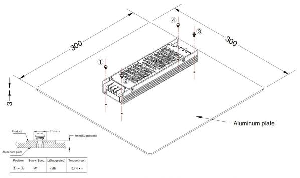
1. In order to meet the "Derating Curve", the product testing must be installed onto an aluminum plate. The size of the suggested aluminum plate is shown as above. And for optimizing thermal performance, it is necessary to apply thermal grease on the bottom of the product.
