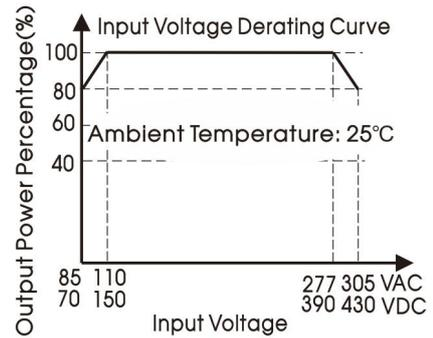
Note: ① With an AC input between 85 - 110VAC/277 - 305VAC and a DC input between 70 - 150VDC/390 - 430VDC, the output power must be derated as per temperature derating curves;
