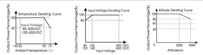
Note: 120-140VDC the output power must be derated as per the temperature derating curves;
